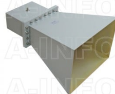
LB-1150-10-C-NF Standard Gain Horn Antenna 0.64-0.96GHz 10dB Gain N Type Female
